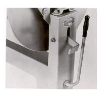
B. To dump mix from drum, stop paddles, move drum latch up and pull dump handle down. Always use caution when dumping mix.
