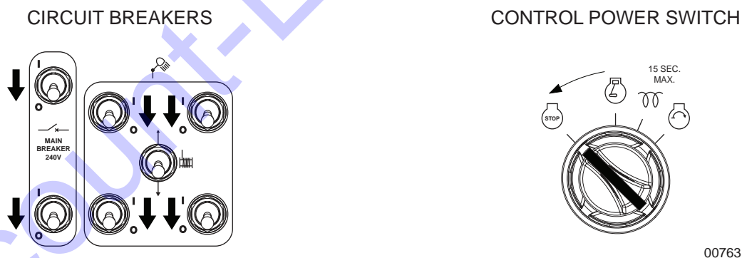
Figure 14 - Breakers and Control Power Switch
