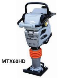
Weight lbs (kg) - 141 (64) Shoe Width in (mm) - 10.4 (265) Engine Option - Honda GX100 Impact Force lbs (kN) - 3,064 (13.6)
