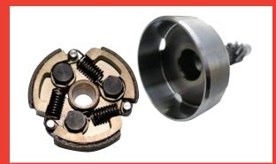
Cam-type Clutch ensures optimum contact between the composite shoes and the drum to eliminate slippage and prolong service life.
