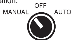
Figure 12. Manual-Off-Auto SW. (Manual Position)
