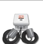
All MQ 115V 1Ø pumps are designed with internal thermal overload protection and do not require extra electrical protection, however, the **CB3 control box** is offered for convenient ON/OFF/AUTO and float switch operations. The CB3 comes with two SW1WOPA Float switches.
