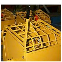
C. Always grease drum seals (at both ends) as recommended in the maintenance chart. The grease purges dirt, prolonging bearing life.
