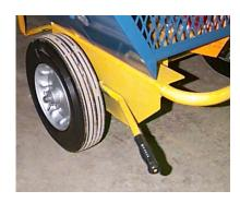
B. To dump mix from drum, stop paddles and pull dump handle down. Always use caution when dumping mix.
