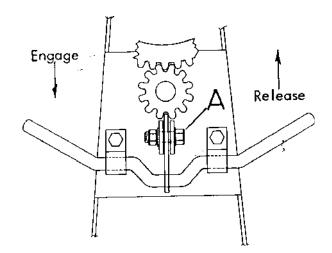
To prevent accidental discharge, never release brake without holding the handwheel firmly. Do not attempt to grab handwheel to stop an accidental discharge, serious injury could result. Always make sure that the brake is fully engaged after discharge of concrete and before reloading drum.
