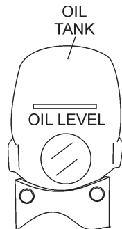
Figure 9. Oil Tank (Front View)
