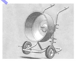
**14.** Mount each mixer paddle inside the assembled drum with the pointed end facing downwards. Also the V-shaped bend in the mixer should pointed in the direction of the drum rotation (clockwise). Use the M8 x 20 mm Hex bolt washer and hex flange nut to secure the unit to the lower mounting holes.
