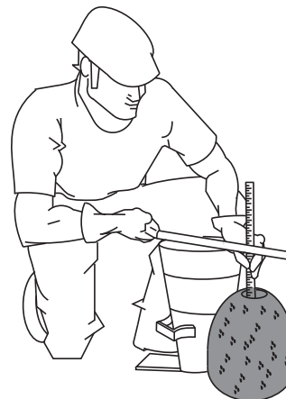
Figure 41-F. Slump Test (Measurement)
