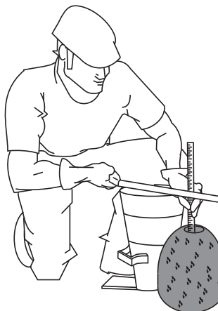
Figure 38-F. Slump Test (Measurement)
