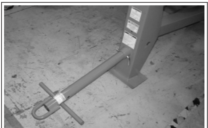
Draw Bar at Mid position for Towing
