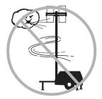
Do not raise the mast when wind speeds may exceed 62 mph / 100 km/h. Do not alter or disable machine components that in any way affect safety and stability.
