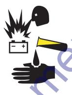
Batteries contain acid. Always wear protective clothing and eye wear when working with batteries.
