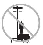
Do not raise the mast to the vertical position unless all outriggers are properly deployed, the foot pads are in firm contact with the ground and the machine is level.
