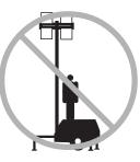
Do not raise the mast to the vertical position unless all outriggers are properly deployed, the foot pads are in firm contact with the ground and the machine is level.
