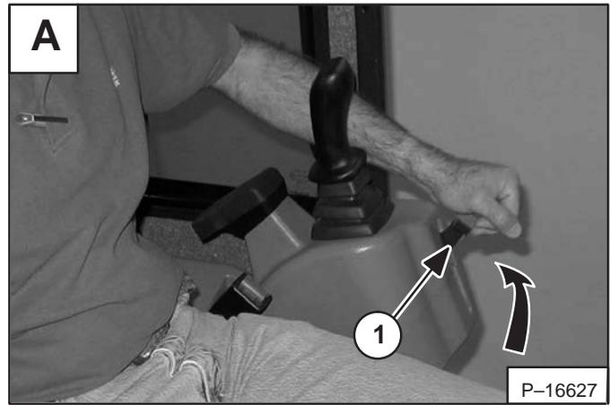
Lower the console before operating the excavator.
