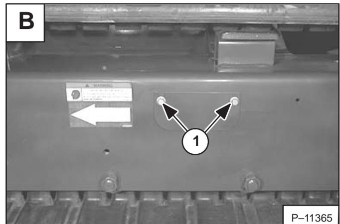
Add grease to the fitting (Item 1) [C] until the track tension is correct.
