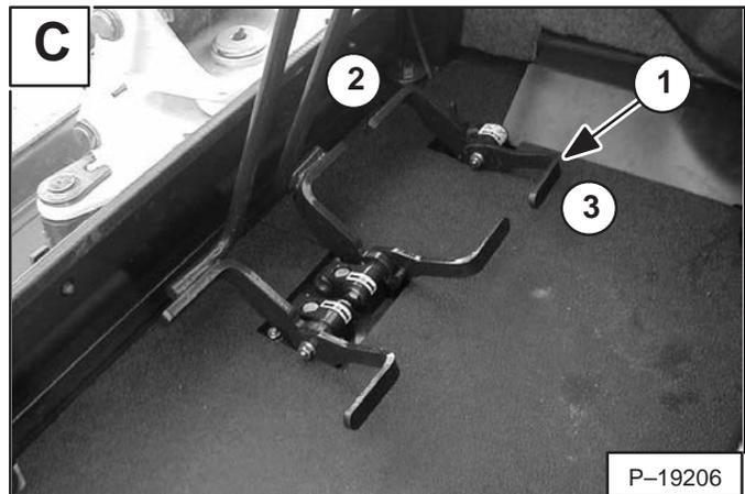
**NOTE: The purpose of the boom swing pedal is to offset the boom with respect to the upperstructure for digging close to a structure [D].**
