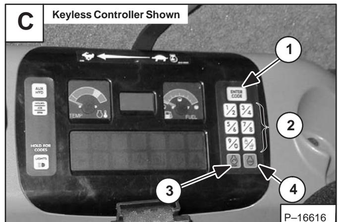
Press the STOP Button (Item 4) **[C]** to stop the engine.
