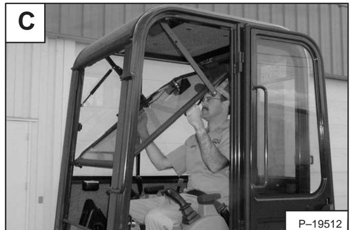
Hold the bottom of the window up and lock the two window latch pins. Make sure that the pins are secured to hold the window up **[D]**.
