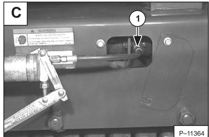
Use tool MEL-1560 (Item 1) [D] to loosen the bleed fitting (Item 2) [D] to release tension from the track.
