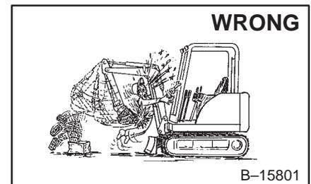
⚠ Always lower the bucket and blade to the ground before doing any maintenance.
