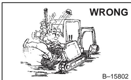
⚠ Stop, cool and clean engine of flammable materials before checking fluid.
