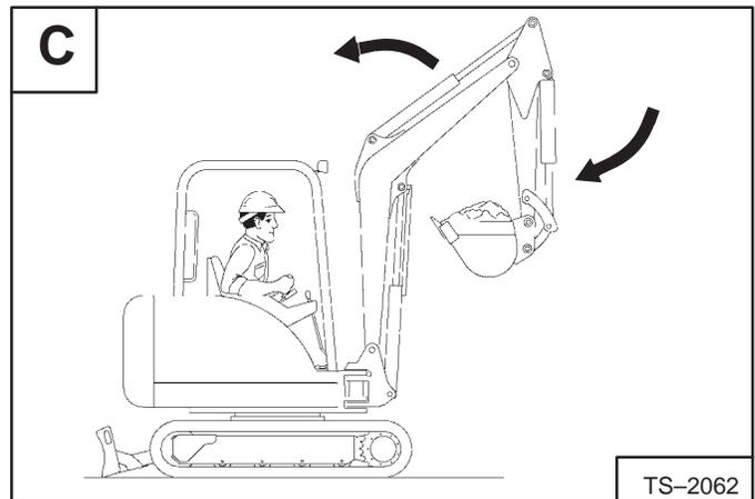
Extend the arm and uncurl the bucket to dump the material into a pile or truck [D].
