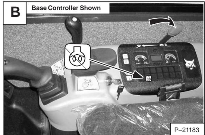
Turn the key to START **[C]**. If preheating is required, the glow plugs will automatically cycle and the remaining preheat time (in seconds) will show in the LCD. (Preheat icon will be ON **[B]**).
