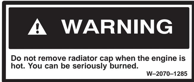
When the engine is cool, loosen and remove the radiator cap (Item 1) [A].
