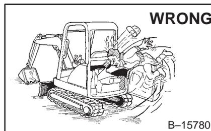
⚠ Keep body, jewelry and clothing away from moving parts, electrical contacts, hot parts and exhaust.
