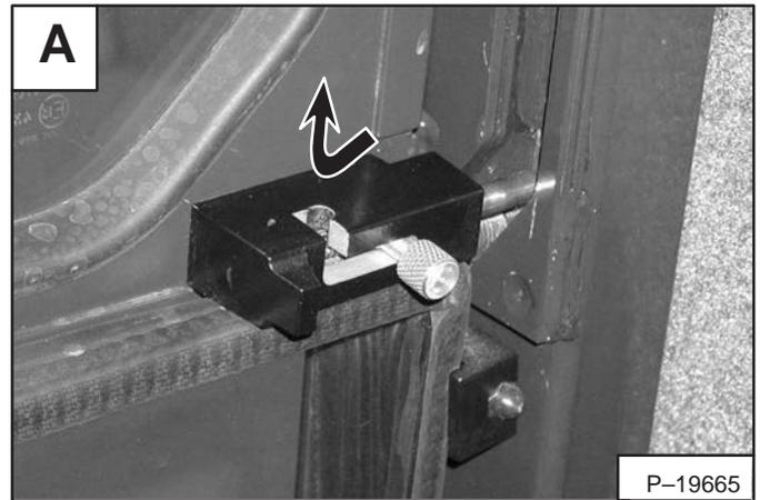
Turn the two top latches (Item 1) **[B]** to the unlocked position.
