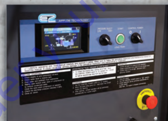
1 | Digital Touch Screen Control with Start button & Pressure Selector switch
