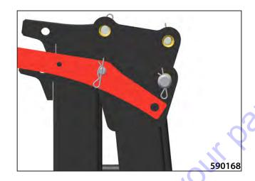
Remove the cotter pins of the rear pins of the ROPS frame.
