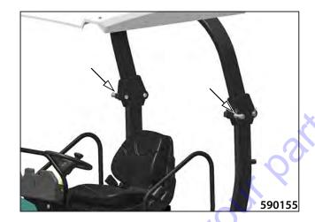
Put the fixture on the outside of the frame and install the front pins of the ROPS frame from the outside of the ROPS frame.
