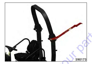
Remove the cotter pins of the rear pins of the ROPS frame. Rotate the ROPS frame fixture.
