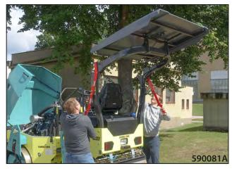
Remove the cotter pins on the front pins of the ROPS frame. Remove the front pins of the ROPS frame.
