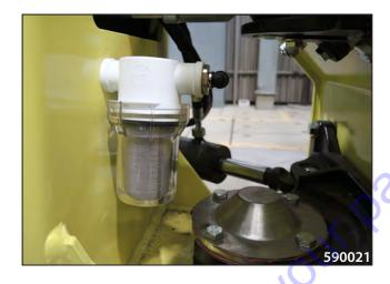
Remove and clean the sprinkler sieves.
