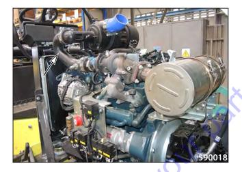
Check the cooling circuit for leakage. Check the hoses for damage and missing hose clips. When hoses are cracked or hardened, replace them for new ones.
