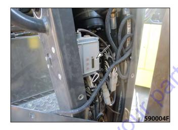
Switch over with the MODE button (1) until  $^{\circ}\text{C}$  appears on the display.
