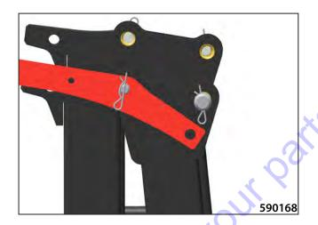
Remove the cotter pins of the rear pins of the ROPS frame. Take out the ROPS frame fixtures.
