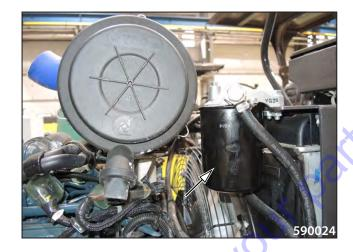
Lubricate the seal rings of the new filters with oil.
