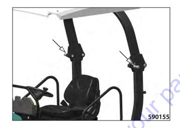
Put the fixtures on the outside of the frame and install the front pins of the ROPS frame.
