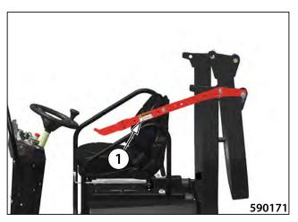
Using the ROPS frame fixture raise the frame completely.
