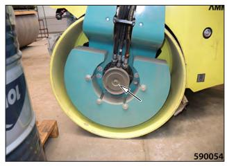
Mount a brake disc on the front drum travel hydraulic motor. Tighten the screw by half a turn.
