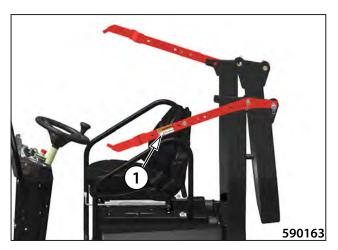
Using the ROPS frame fixtures raise the frame completely.
