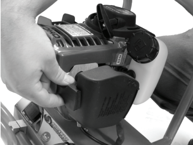
Step 1 – Remove carburetor cover by pressing clips.
