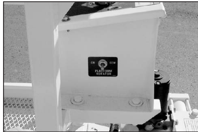
Figure 6.6—Upper Control Panel Side
