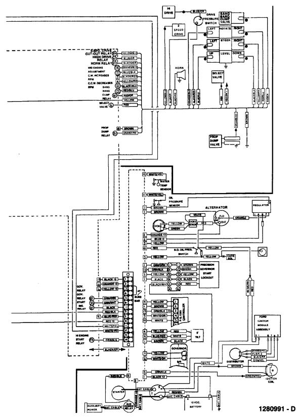
Figure 3-18. Wiring Diagram - Standard (Ford Dis Engine W/ Hydraulic Controls) (Sheet 2 Of 2).
