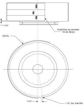
Figure 2-49. Capacity Indicator Dial
