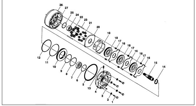
Figure 2-39. Swing Brake Assembly - Mico (Machines Built Prior To May 1992).
