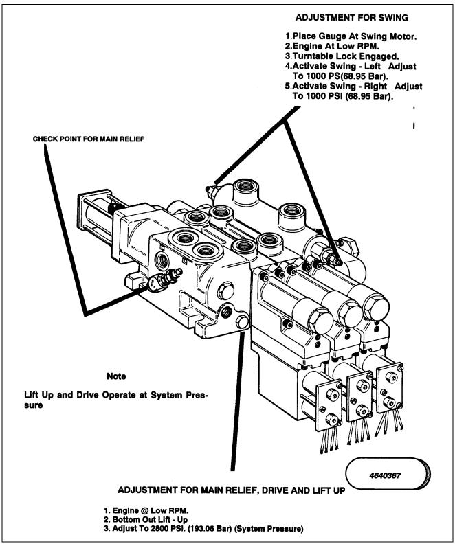
Figure 2-12. Racine Proportional Valve Pressure Setting.(Machines Built Prior To Mid 1987) (Sheet 1 of 2)
