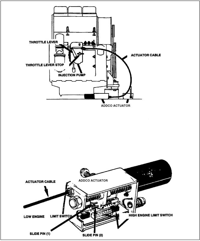
Figure 2-10. Addco Actuator Adjustments, F3L912.
