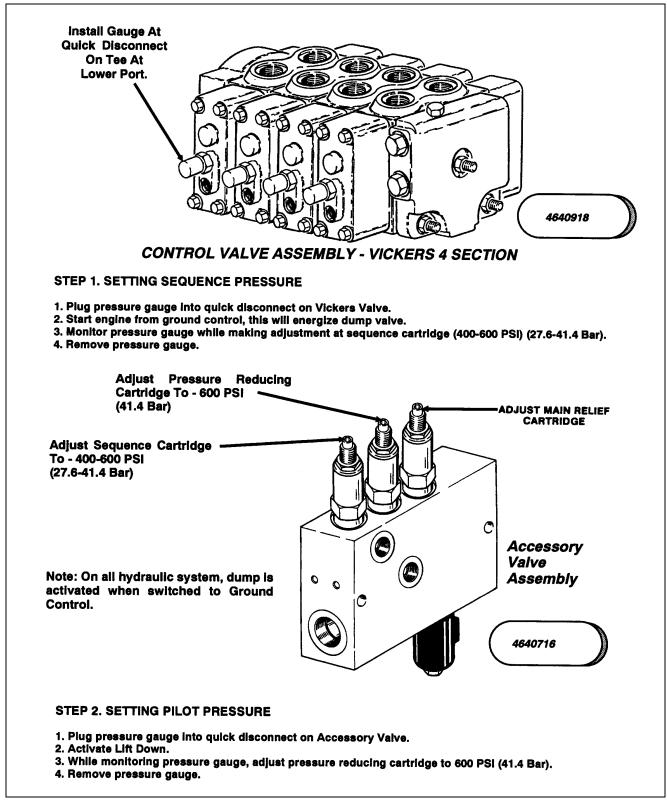
Figure 2-24. Vickers All Hydraulic Machines Pressure Settings (Sheet 1 of 4).
