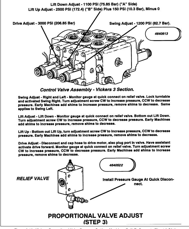
Figure 2-16. Vickers Proportional Valve Pressure Setting, Machines Built To Present. (Sheet 3 Of 4)
