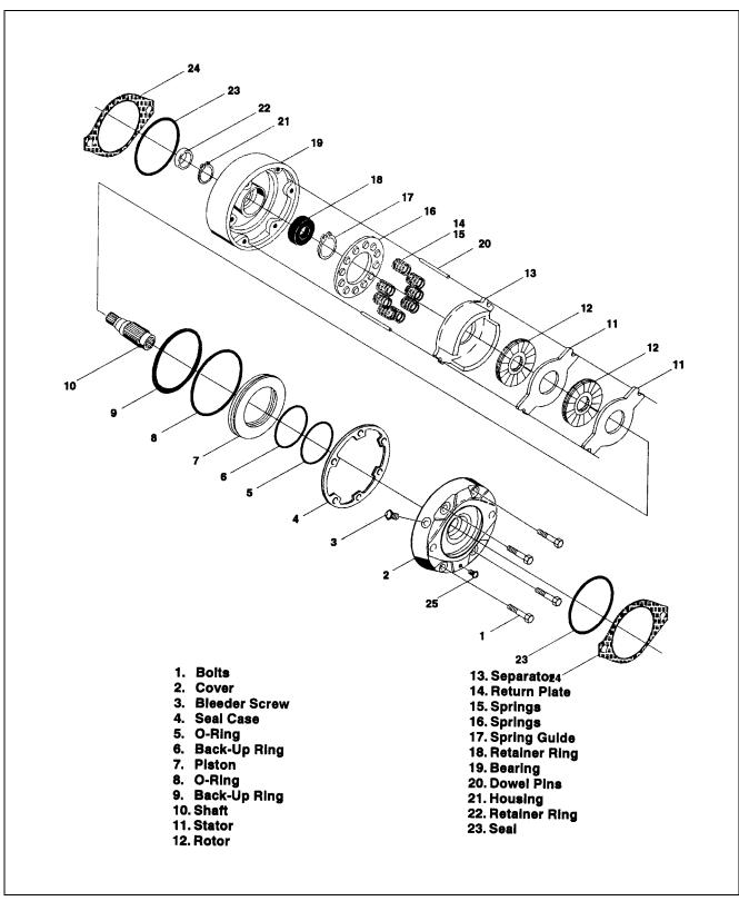
Figure 2-43. Drive Brake, Mico. (Machines Built From May 1992 To Machine S/N 33476)
