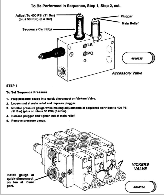
Figure 2-18. Vickers Proportional Valve Pressure Setting, Machines Built Prior To 1989 With Accessory Valve. (Sheet 1 of 4).
