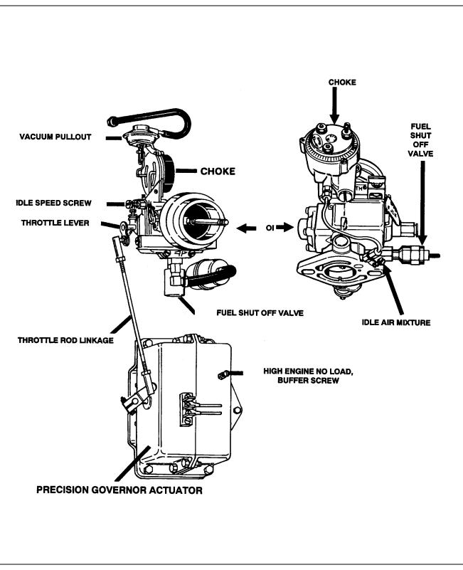
Figure 2-6. Precision Governor Adjustment, Ford. (Sheet 1 of 2).
