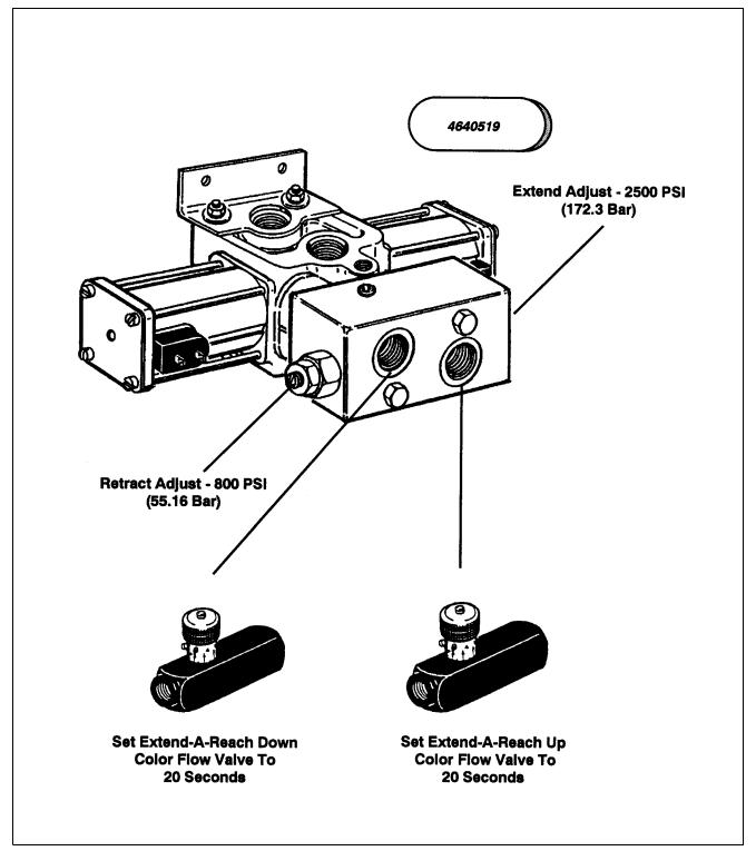
Figure 2-30. Extend-A-Reach Valve Pressure and Speed Settings Model 40+6.
