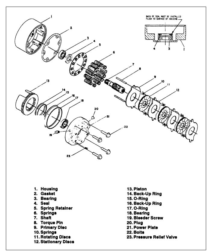
Figure 2-41. Swing Brake Assembly - Ausco (Machines Built Prior to May 1992).
