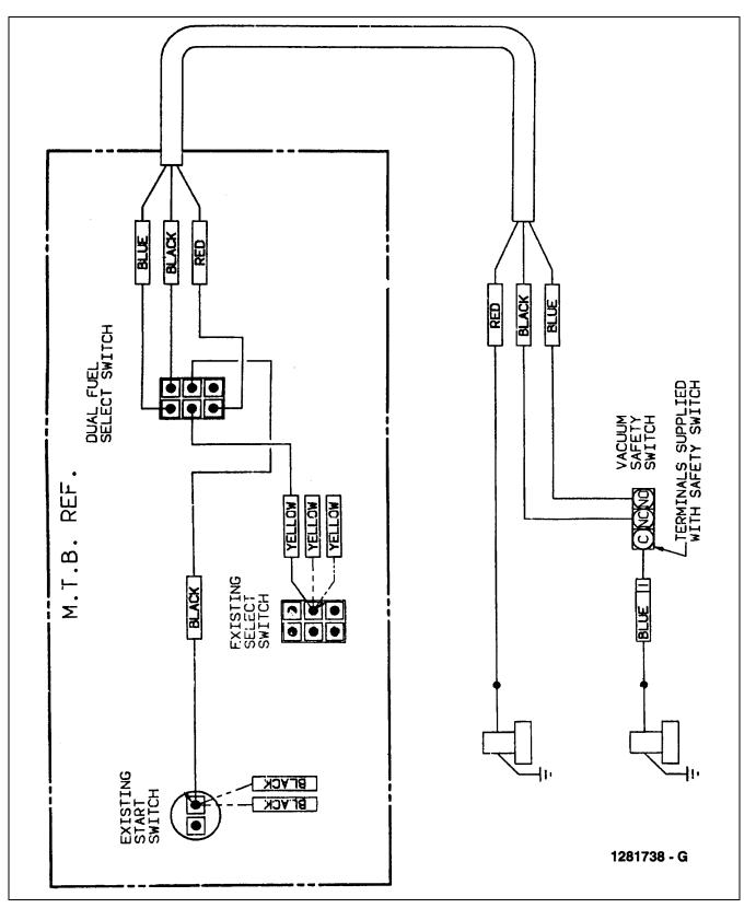
Figure 3-1. Wiring Diagram - Dual Fuel (Ford Or Wisconsin)
