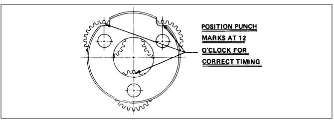
Figure 2-38. Torque Hub Carrier Timing.
