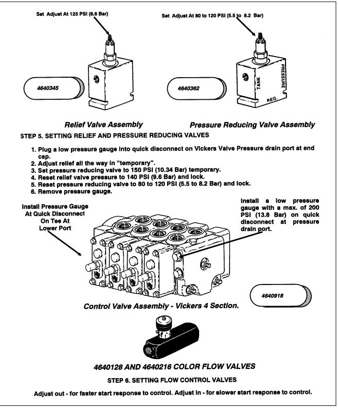
Figure 2-27. Vickers All Hydraulic Machines Pressure Settings (Sheet 4 of 4).
