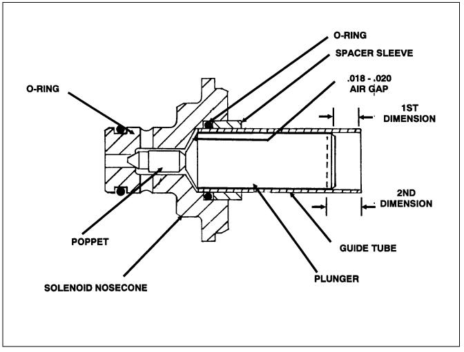
Figure 2-31. Racine Proportional Air Gap Adjustment, Machines Built Prior To Mid 1987.
