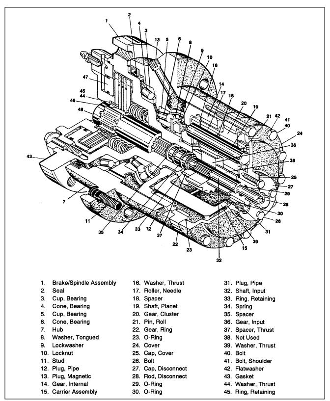
Figure 2-37. Torque Hub 4/WD.
