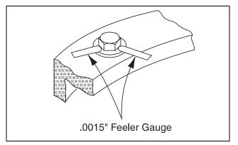
Figure 2-33. Swing Bolt Feeler Gauge Check.
