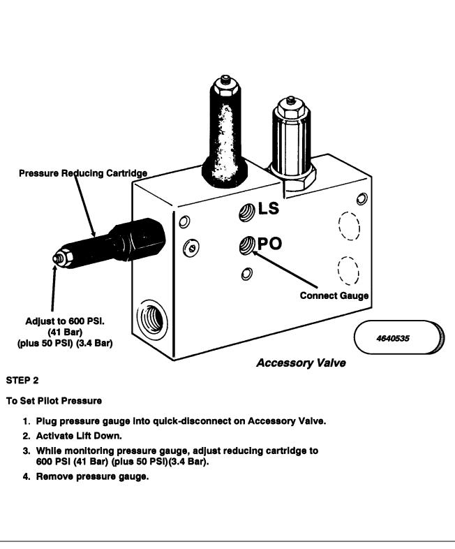
Figure 2-19. Vickers Proportional Valve Pressure Setting, Machines Built Prior To 1989 With Accessory Valve. (Sheet 2 of 4)
