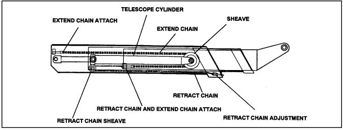
Figure 2-1. Typical Three Section Boom Assembly.
