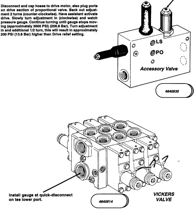
Figure 2-21. Vickers Proportional Valve Pressure Setting, Machines Built Prior To 1989 With Accessary Valve. (Sheet 4 Of 4)
