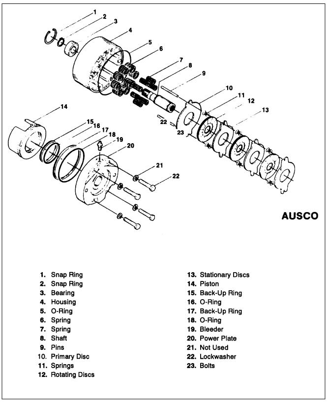
Figure 2-42. Drive Brake, (machines Built Prior to May 1992).
