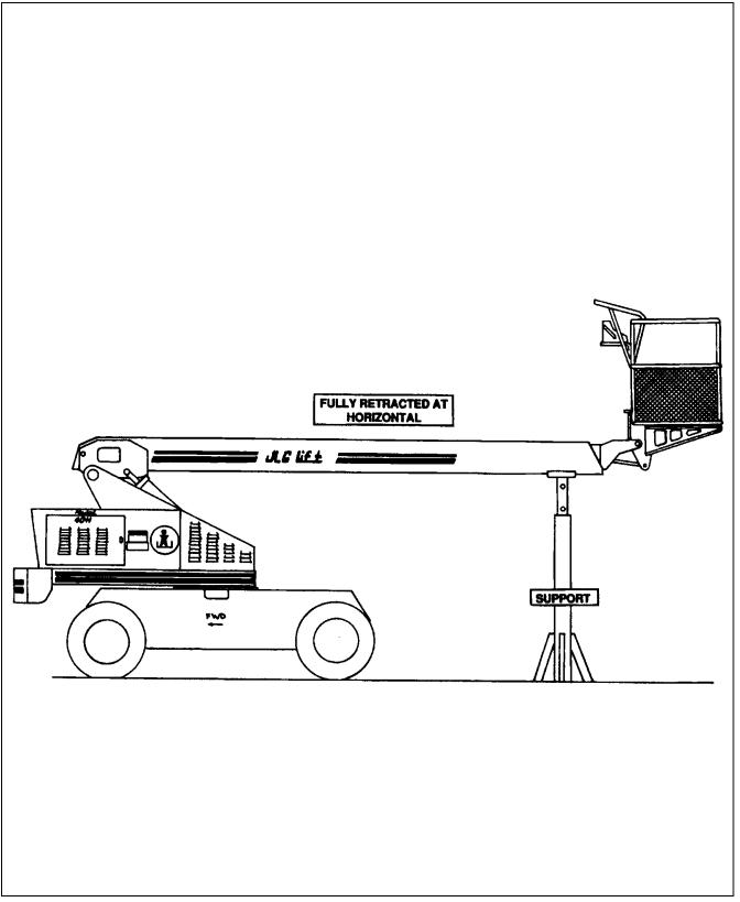
Figure 2-2. Boom Positioning and Support, Cylinder Repair.
