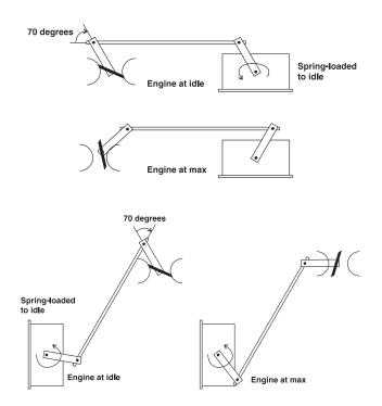
The needed travel of the carburetor determines how far out the Actuator arm the rod is to be attached. Inmost cases, The carburetor should be moved from closed to above 10 degrees from full open as the Actuator is moved min. to max. THEN ALTER THE LENGTH OF THE ROD SLIGHTLY (PERHAPS.030"), SO THAT THE ACTUATOR IS JUST OFF ITS INTERNAL STOP, AND IS PULLING THE BUTTER-FLY AGAINST ITS STOP. This insures that the carburetor can fully close to idle on load dumps, minimizing over speeds.
