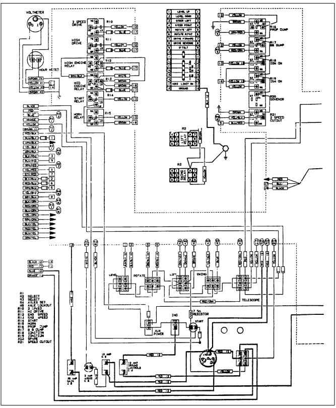
Figure 3-7. Wiring Diagram - Standard (Deutz F2I511/f3I912 & Wisconsin Engine W/ Standard Controls) (Sheet 1 Of 2).
