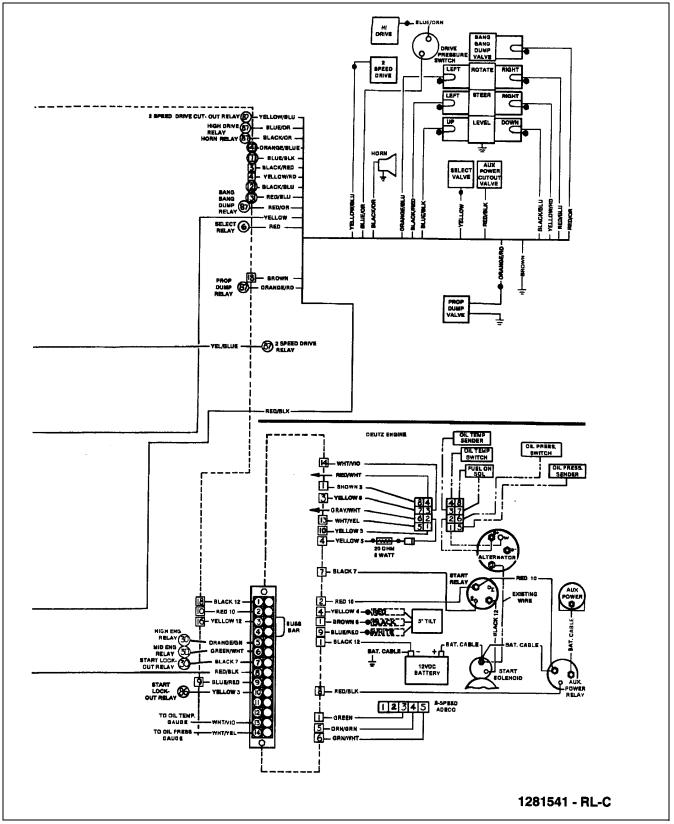
Figure 3-14. Wiring Diagram - Standard (Deutz F3I1011 Engine W/ Hydraulic Controls) (Sheet 2 Of 2).
