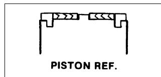
Figure 2-3. Poly-Pak Seal Installation.
