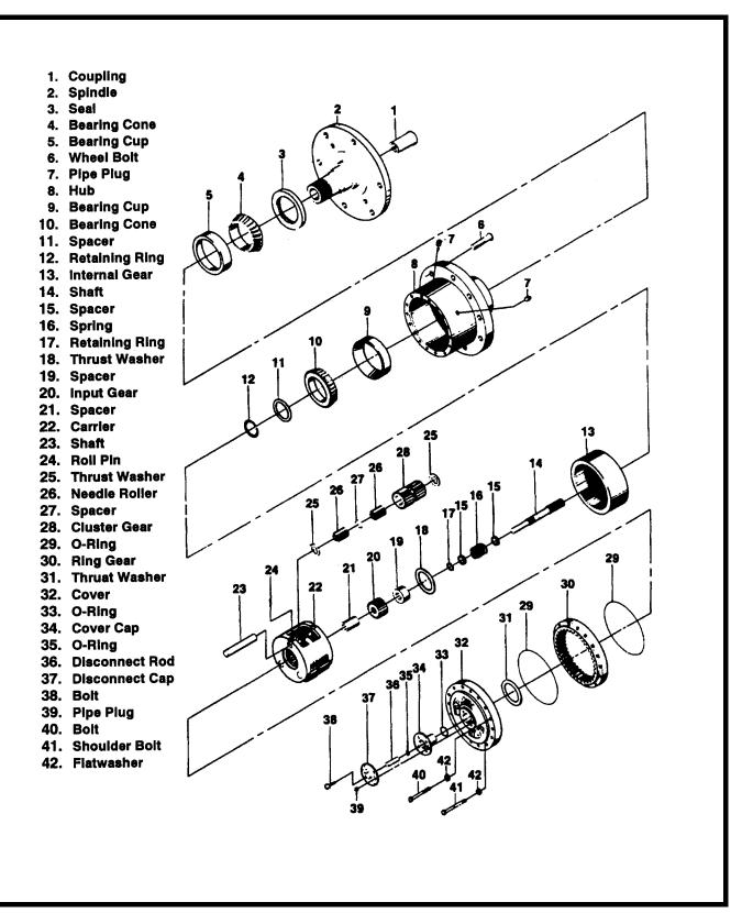
Figure 2-36. Torque Hub Assembly, 2/WD.
