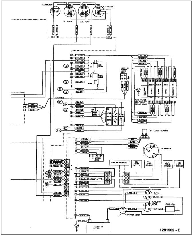
Figure 3-12. Wiring Diagram - Standard (Deutz F3I1011 Engine W/ Standard Controls) (Sheet 2 Of 2).
