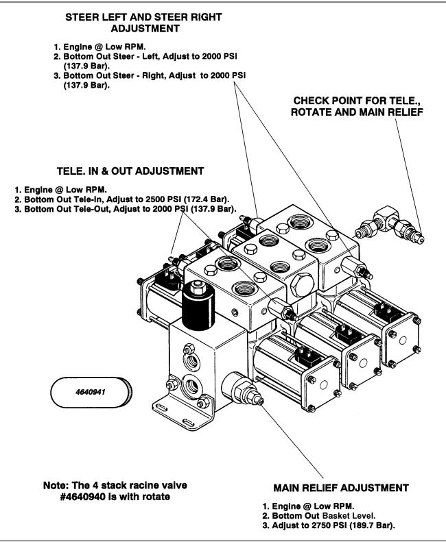
Figure 2-29. Solenoid Valve Pressure Settings, Machines Built from 1995 To Present. (Sheet 2 of 2)
