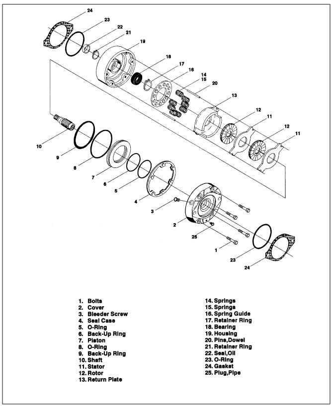
Figure 2-45. Drive Brake, Mico. (Machines Built From S/N 33476 To Present)
