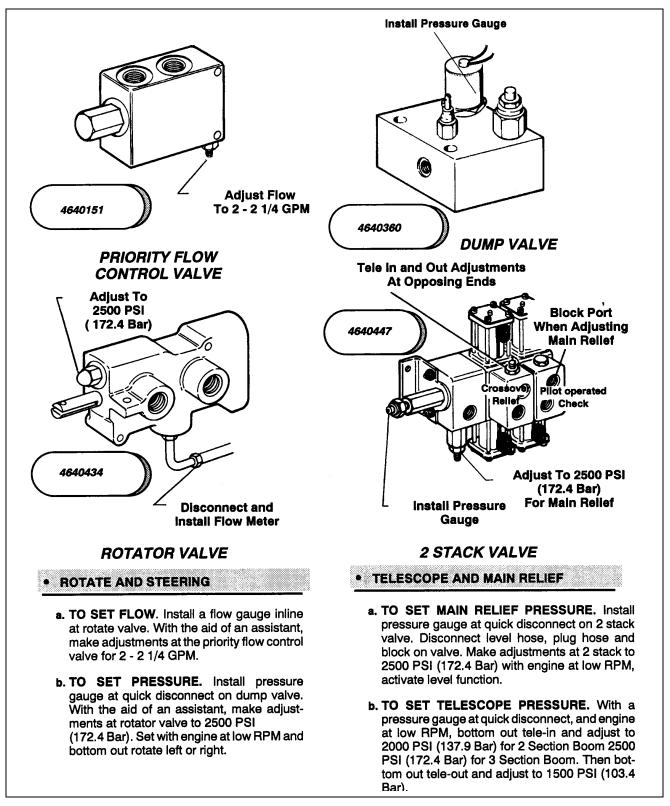
Figure 2-23. Pressure And Flow Settings (Machines Built Prior To May 1992 With Steering Wheel).
