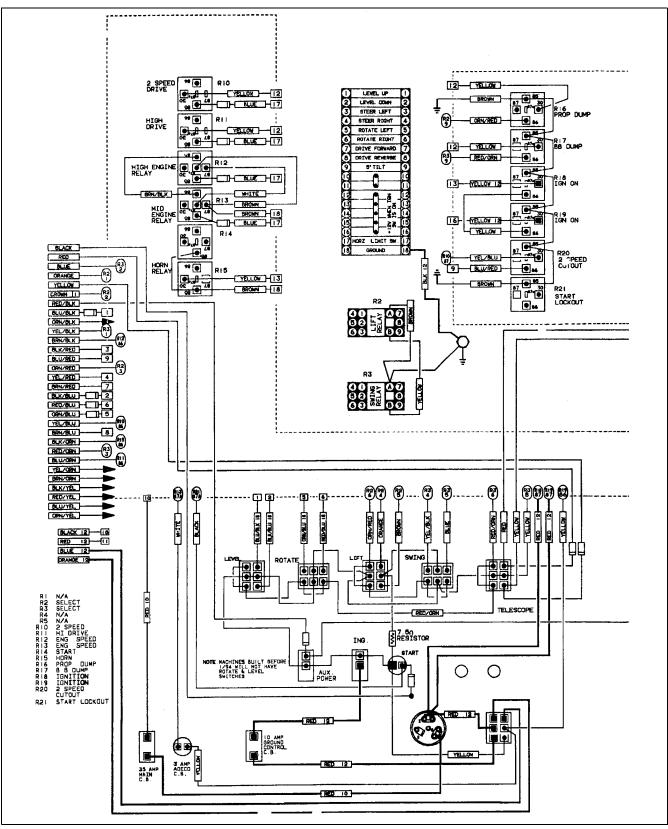
Figure 3-11. Wiring Diagram - Standard (Deutz F3I1011 Engine W/ Standard Controls) (Sheet 1 Of 2).
