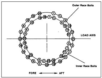
Figure 2-35. Swing Bearing Torquing Sequence.
