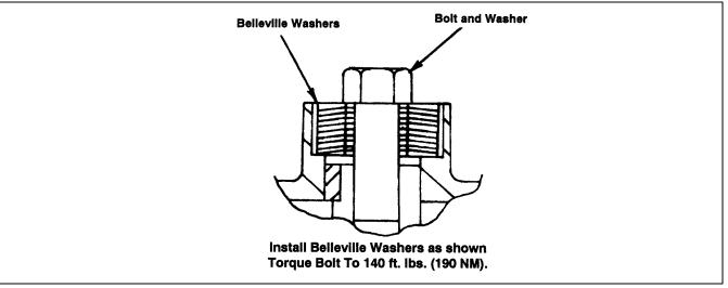
Figure 2-47. Basket Rotator Brake.
