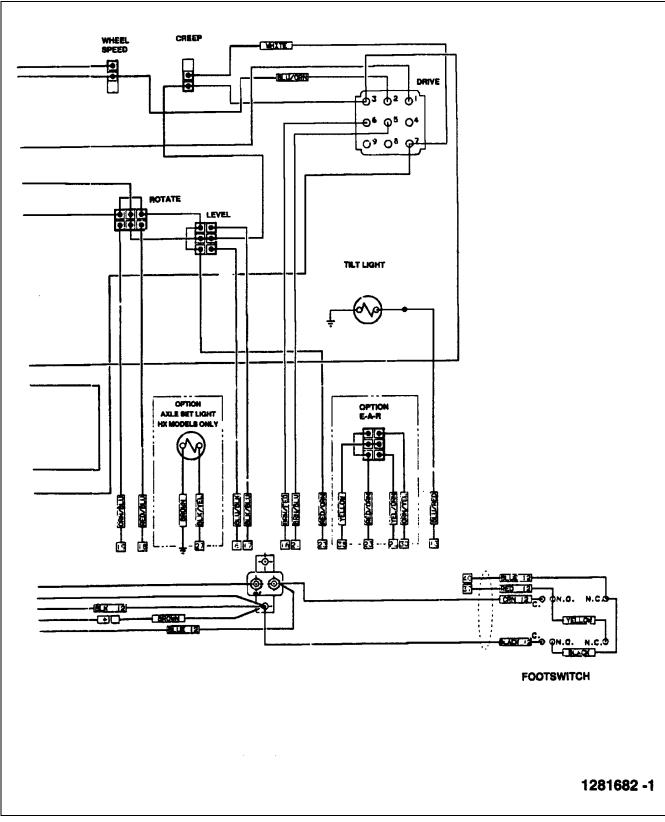
Figure 3-6. Wiring Diagram - Platform Console Standard (Sheet 2 Of 2).
