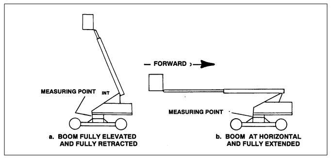
Figure 2-32. Swing Bearing Tolerance Boom Placement.
