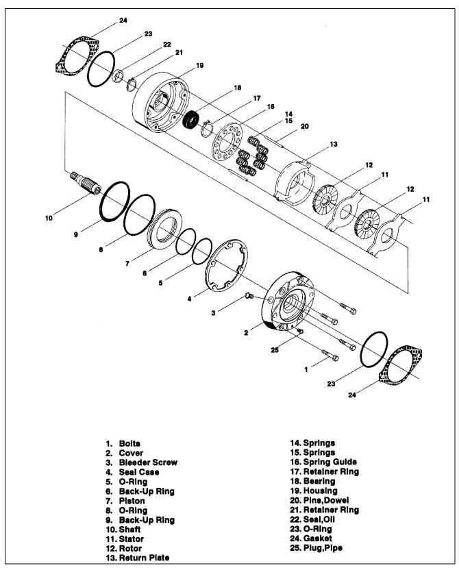
Figure 2-46. Swing Brake, Mico. (Machines Built From S/N 33476 to Present)
