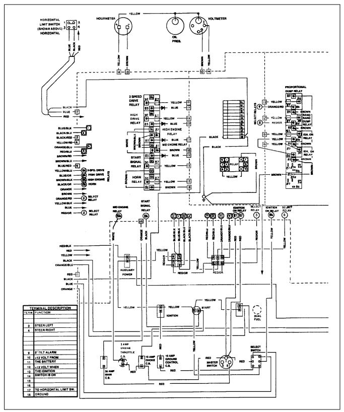
Figure 3-9. Wiring Diagram - Standard (Deutz F2I511/f3I912 & Engine W/ Hydraulic Controls) (Sheet 1 Of 2).
