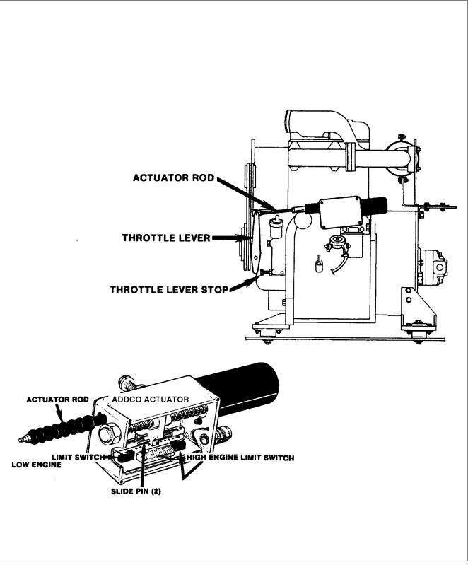
Figure 2-8. Addco Actuator Adjustments, F2L511.
