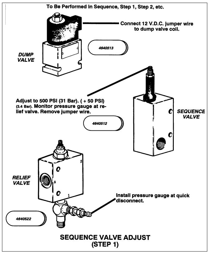
Figure 2-14. Vickers Proportional Valve Pressure Setting, Machines Built To Present (Sheet 1 of 4)
