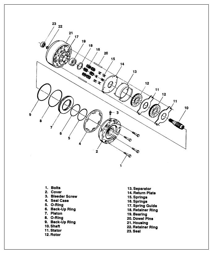
Figure 2-44. Swing Brake, Mico. (Machines Built From May 1992 To Machine S/N 33476)
