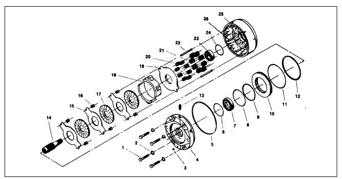
Figure 2-40. Drive Brake Assembly - Mico (Machines Built Prior To May 1992).
