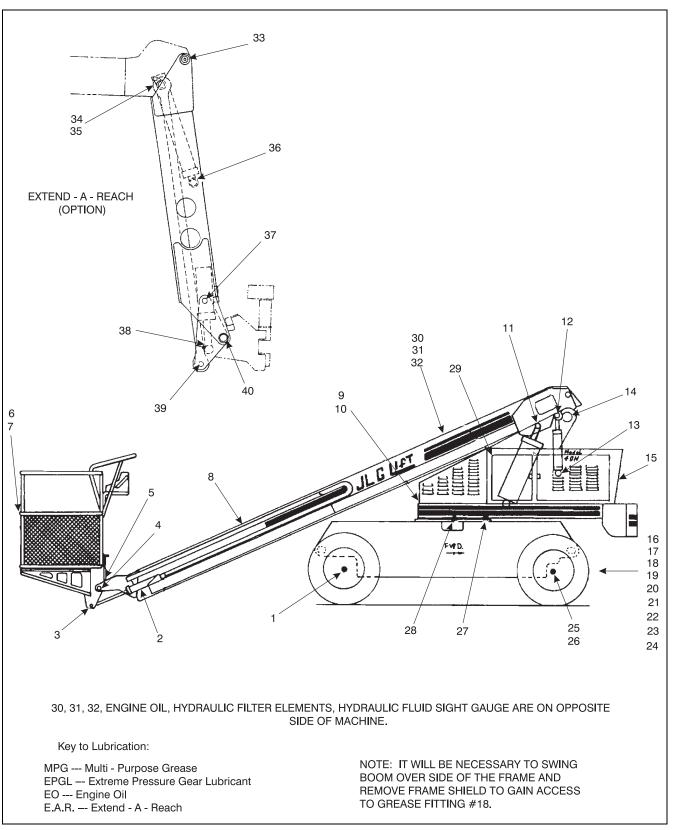
Figure 1-2. Lubrication Chart. (Sheet 1 of 2)
