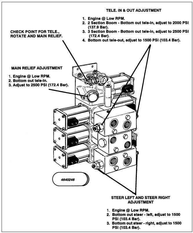
Figure 2-22. Solenoid Valve Pressure Settings. (Machines Built Prior To 1992 With Steering Wheel)
