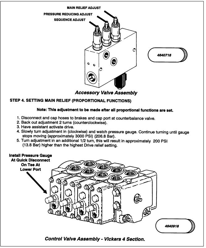
Figure 2-26. Vickers All Hydraulic Machines Pressure Settings (Sheet 3 of 4).
