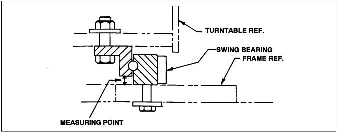
Figure 2-34. Swing Bearing Tolerance Measuring Point.
