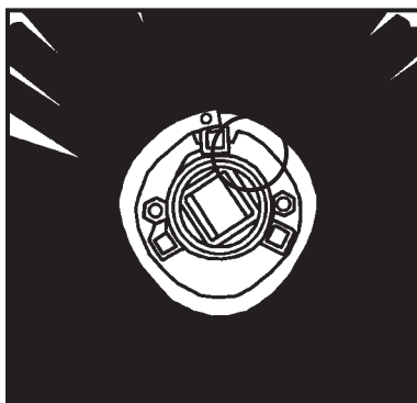
FIGURE 4 Improper Placement of Drive Pins (Circled)
