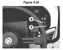
Press and hold park brake test switch (8, Figure 5-20) and move propulsion control (14, Figure 5-21) towards the Forward position to attempt machine movement. If the parking brake system is functioning, the machine will not move. If machine moves, contact service personnel and do not operate machine.
