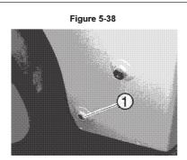
3. Remove drain plug (1, Figure 5-38) and fill plug (1, Figure 5-39) and drain the hydraulic tank. Dispose of used hydraulic oil in accordance with local guidelines.
