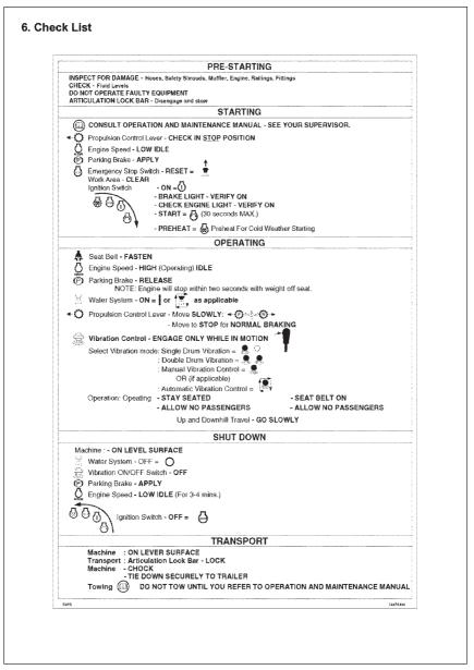
DD-24/30/28HF/34HF Vibratory Asphalt Compactors
