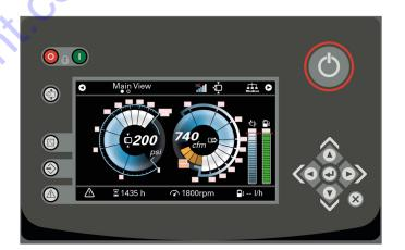
Histogram: The new Xc4004 gives enables Performance Monitoring System by creating onboard histograms of major parameters like FAD, Engine Load, Highest element temperature, Vessel Pressure, Engine RPM, Fuel Rate etc...
