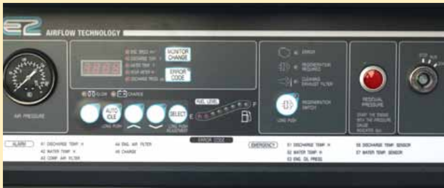
Diagnostic Control Panel — Monitors low fuel level, battery, fuel filter, engine oil filter, water temperature, compressor air filter, oil pressure, discharge air temperature and auto idle.
