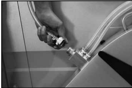
Fig. 5 Unscrew Hose Fitting
