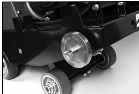
Fig. 8 Pull Out Outer Flange
