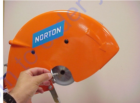
Blade Shaft Bolt Removal
