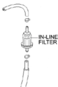
Figure 16. In-Line Fuel Filter
