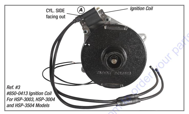
When the ignition coil (A) is installed correctly, the wording "this side out" will actually be facing in towards the machine. The front side of the coil, which will be facing out towards you, will read 'CYL. SIDE'. Coil to magnet gap = .010 inch.
