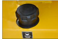
pending plastic water tank eliminates water flow obstructions from rust build-up.
