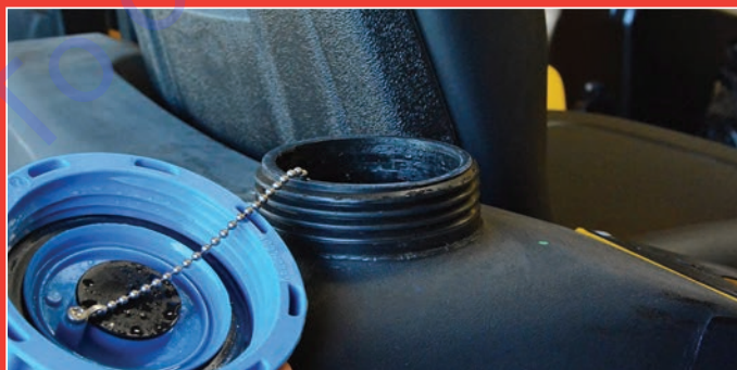
Plastic water tank eliminates rust and pressurized system provides better water flow.
