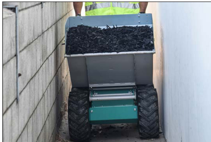
Optional 7 ft 3 steel clip-on tub — TT7 — allows access through narrow 32-inch passageways.
