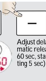
Adjust delay of automatic release (max. 60 sec, standard setting 5 sec)
