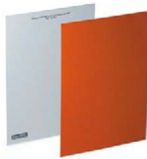
Leica GZM26 target plate For measurements on to poorly reflective surfaces. Two-sided – grey side for shorter distances and brown for longer. Size: 210 x 297 mm. Art. No. 723 385
