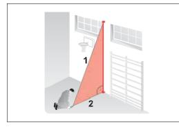
e.g. for measuring building heights or widths. It is helpful to use a tripod when measuring heights that require the measurement of two or three measurements.
