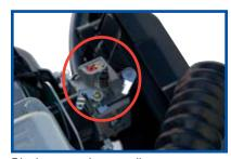
Diaphragm carburetor allows rammer to be laid down in any position without fuel spillage.
