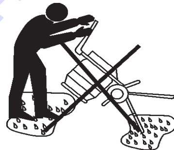
Figure 13. Slippery or Wet Surfaces
