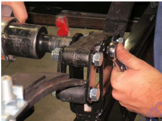
Figure 6. Loosening Axle Hex Nuts
