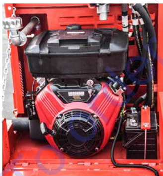
18 HP Vanguard gasoline engine
