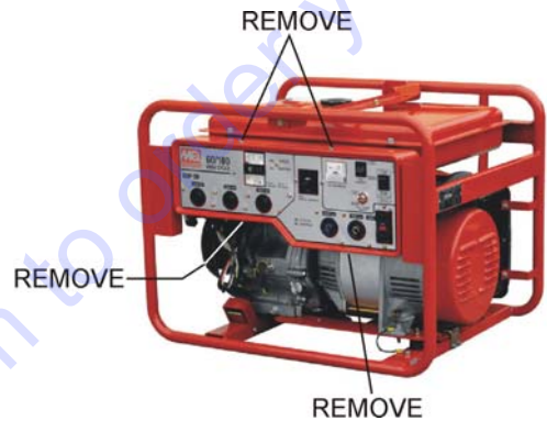
Figure 1. GDP-5H Control Panel Removal
