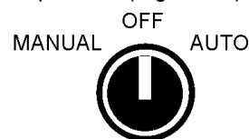
Figure 17. Manual-Off-Auto SW. (OFF Position)
