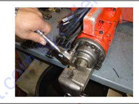
**CAUTION**: Make sure to leave the two bottom bolts and one top bolt for last. Slowly and evenly back the bolts off. This will relieve the tension on the cutter rod return spring.
