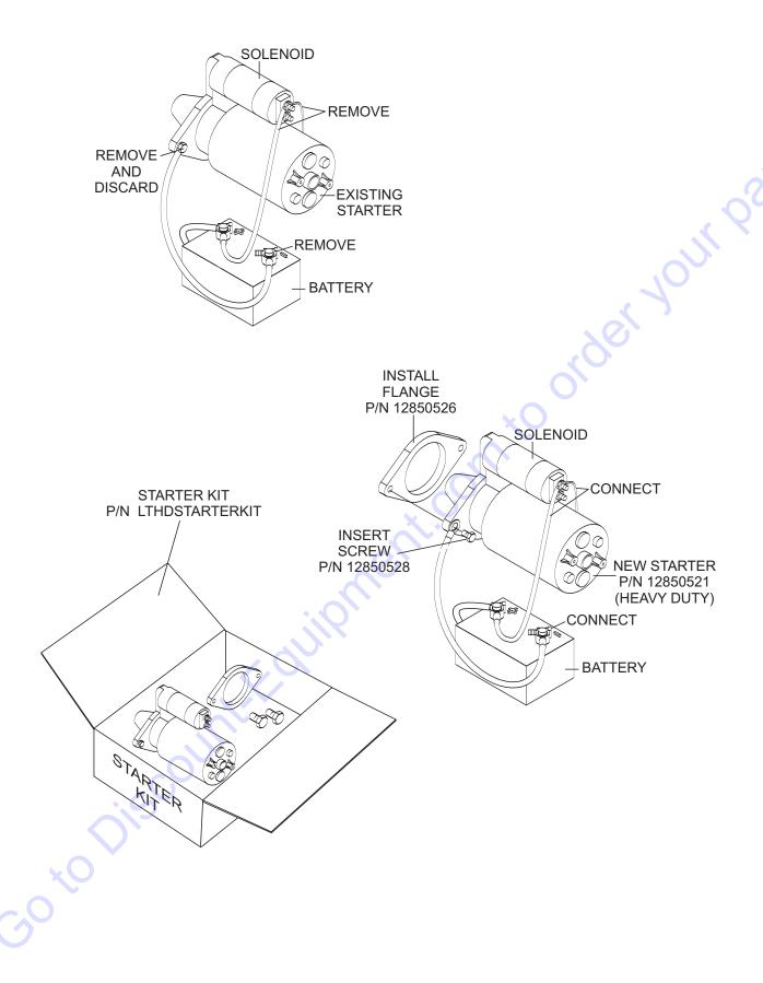
Figure 1. Starter Kit Installation
