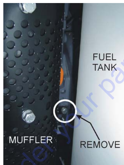
Figure 7. Muffler Bracket Removal
