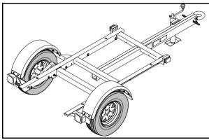
The fixed towbar trailer is equipped with a torsion axle, standard pintle towing eye, tongue mounted jack and trailer lighting system.
