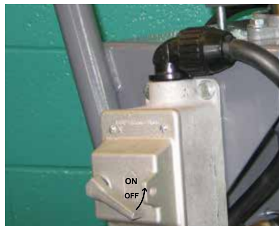
Figure 8. Electric Motor ON/OFF Switch
