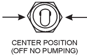
Figure 41. Pumping Switch (No Pumping)
