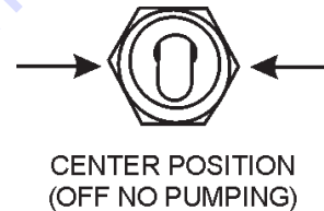
Figure 38. Pumping Control Switch Center Position (No Pumping)
