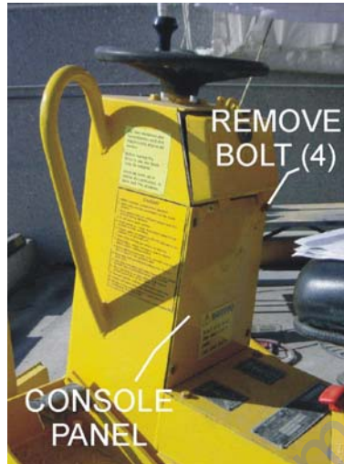
Figure 4. Console Panel Removal
