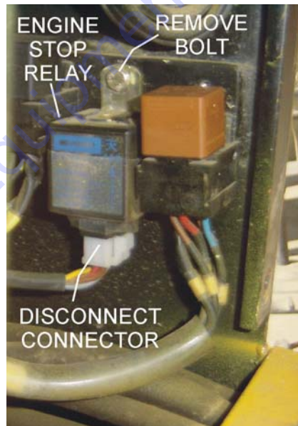
Figure 5. Engine Stop Relay Removal/Installation
