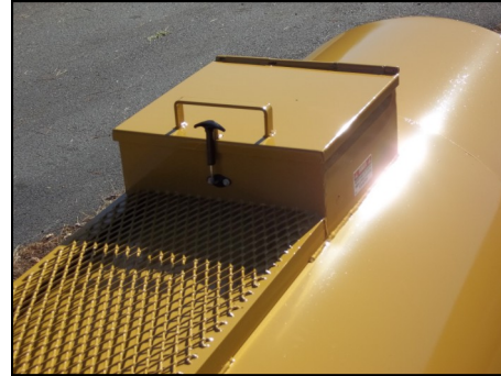
Sealed Man way With Catwalk
