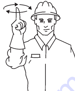
START PUMP SPEED UP
