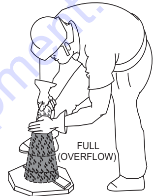
Figure 34-C. Slump Test (Full-Overflow)
