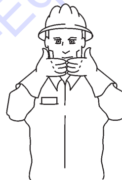
ALL DONE CLEAN-UP
