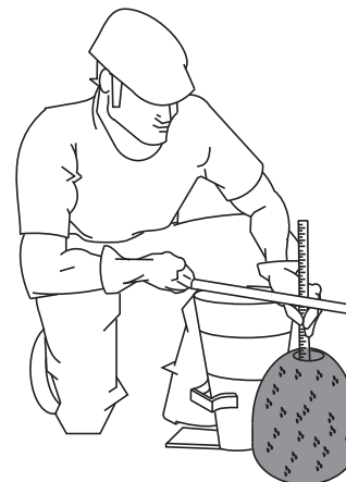
Figure 34-F. Slump Test (Measurement)
